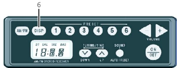
To switch the frequency display to the time display, press the "DISP" key in this condition. (To switch the time display to the frequency display, press the "DISP" key. After the display of station for 1.5 seconds, the display changes to frequency display.)
