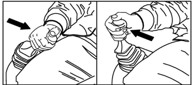
4. When the machine warming up is not sufficient, move the control lever to the stroke end of bucket digging side, and execute more 2 minutes relief operation. And then extend and/or retract the rod of each cylinders several times slowly for the purpose of circulating of warm hydraulic oil. Also operate swing and travel slowly and circulate the warm hydraulic oil.
