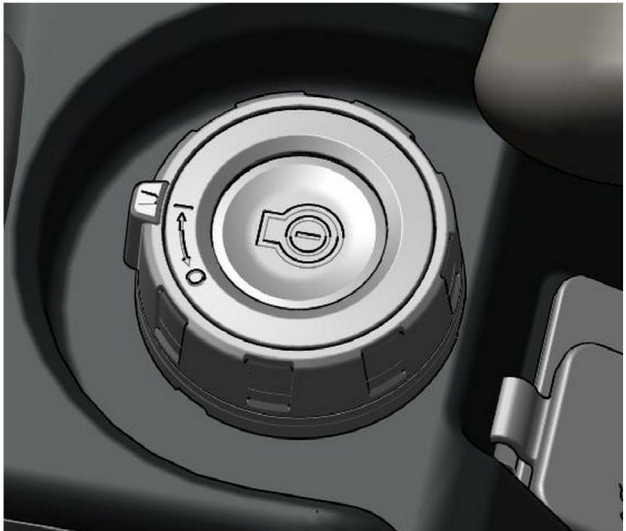
Illustration 145 Engine start switch with integrated MSS indicator
