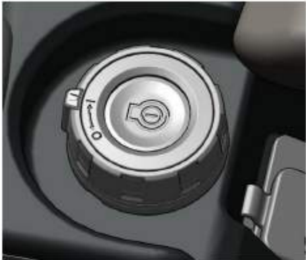
Illustration 190 g06215426 Engine start switch with integrated MSS indicator
